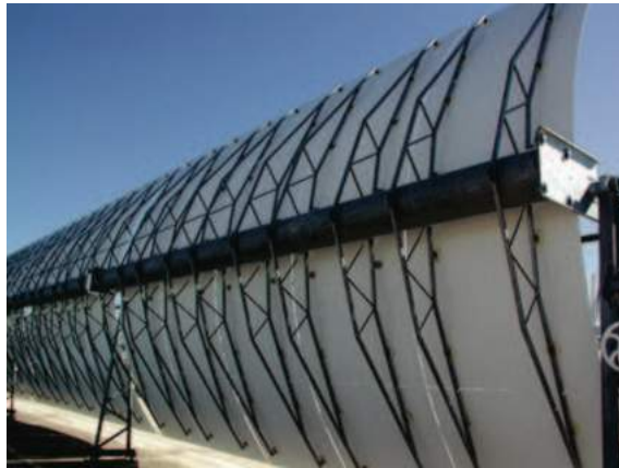
Figura 2.9 – Coletor solar LS-2. Fonte: Parabolic Trough CSP Technology: state of the art and market overview
